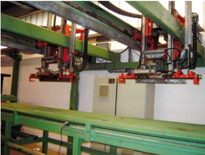
5 robots transport pallet elements to nailing machine pockets (A.S.)
