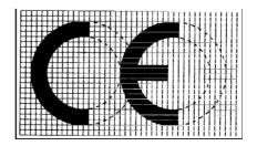
If the CE marking is reduced or enlarged the proportions given in the graduated drawing in paragraph 1 must be respected.
